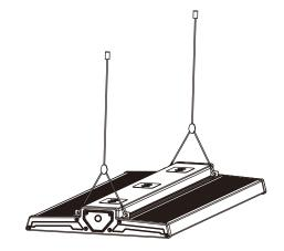
Step 2 Connect ropes with high bay properly and make sure the high bay is hanging straight
